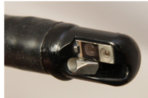
Figure 1: Close-up view of an ERCP endoscope tip.
